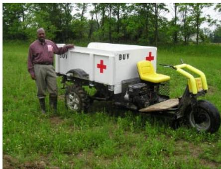
The BUV is a three wheeled vehicle which utilize a 10 horsepower diesel engine and a small pickup truck rear-end wheel assembly. The BUV will be used to transport patients, supplies, and equipment to and from the health center and the reference hospital. And the BUV will be used to generate electricity for the health center. Finally, it can run pumps and grain mills for the village.
